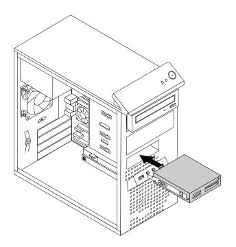
Figure 27. Installing the card reader
